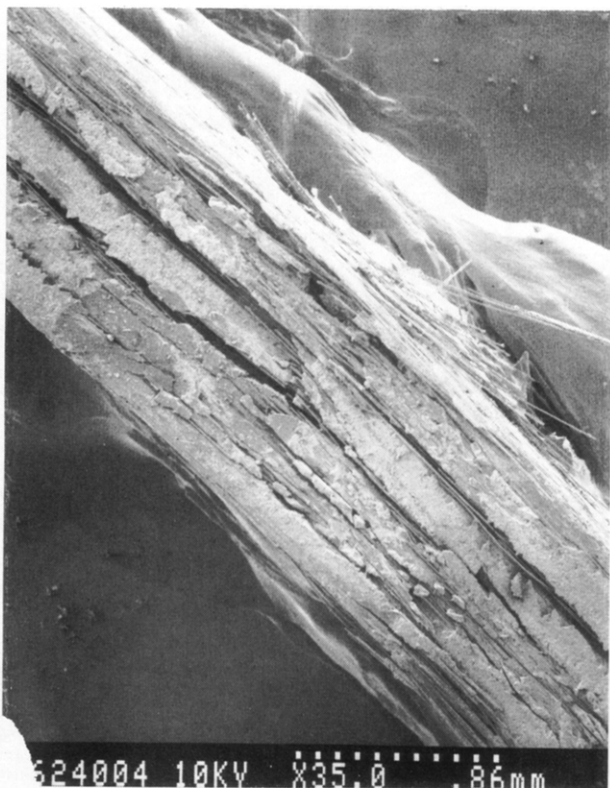
Figure 5. SEM image of fracture side view for 60 wt % of pitch/BN composite annealed at 1200 °C for 3 h.
